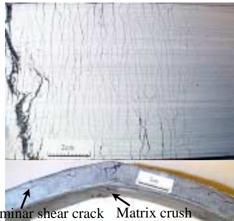
Fig.8 Ultimate State of Specimen Series 5 (2 Layers of ES2, with Spectra fiber V_f=1.5\% )
