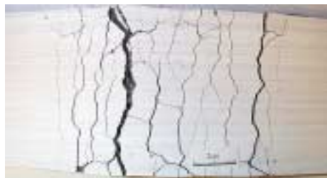
Fig. 9 Ultimate State of Specimen Series 6 (2 Layers of Mesh ES1, with PVA fiber V_f=2.0\% )
