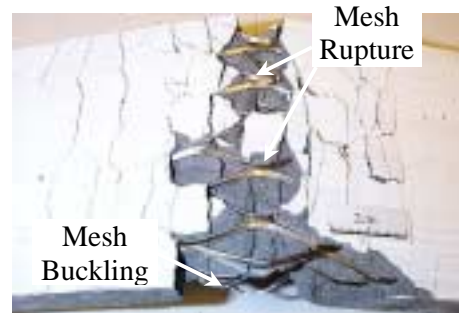
Fig. 4 Ultimate State of Specimen Series 2 (2 Layers of Mesh ES1, w/o fiber)
