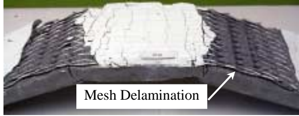
Fig. 5 Ultimate State of Specimen Series 3 (2 Layers of Mesh ES2, w/o fiber)
