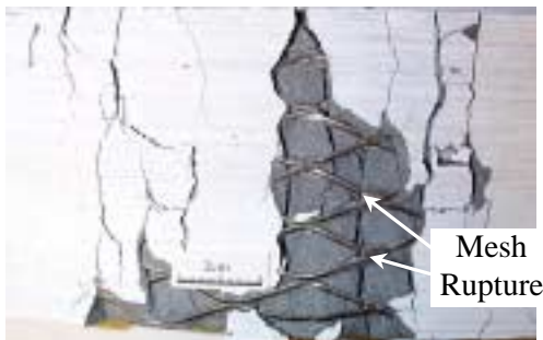
Fig. 3 Ultimate State of Specimen Series 1 (4 Layers of Mesh ES1, w/o fiber)
